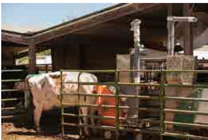
An open-air device measures the methane in the cows’ breath as they eat a treat. (Gregory Urquiaga/UC Davis)
